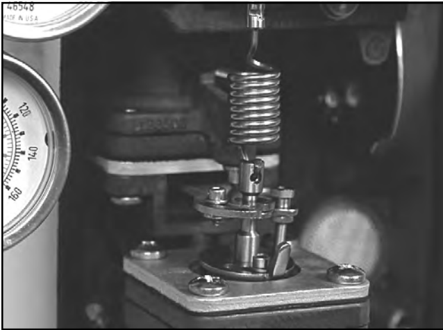
Figure 8: Close-up of Gain Adjustment
