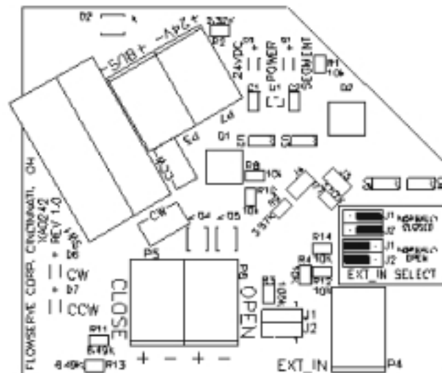
Figure 4 Interface Card: 4-Wire Version XA0242
