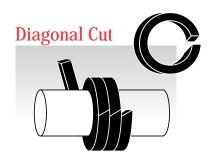
**Press ring** into the bottom of the box and seat gently with tamping tool or split bushing. Rotate shaft after each ring is installed. Stagger joints 180°. Seat rings of foil packing very firmly.
