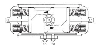
Exhausting the air pressure from Port 1 allows stored energy of the springs to drive pistons inward, turning the pinion clockwise. Air volume on outside of pistons vents through Port 2.
