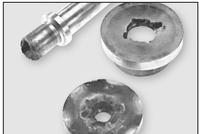
Figure 4: Damage to Trim Parts Caused by Cavitation
