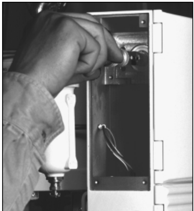
Figure 12: Poppet Guide Installation
