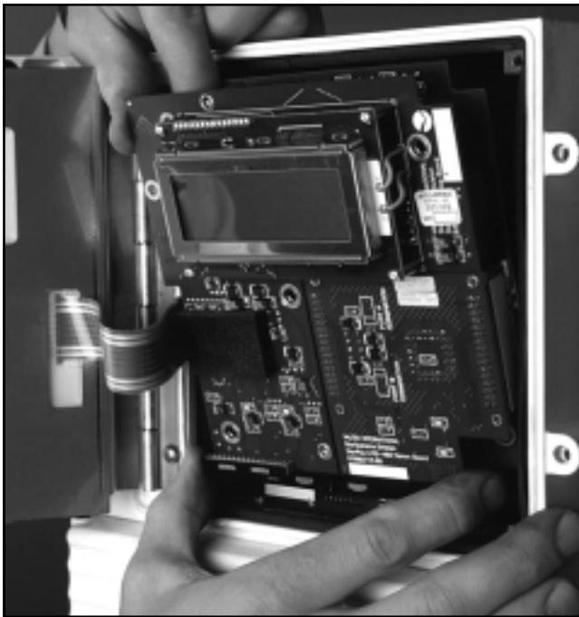
Figure 14: Replacing the Board Stack
