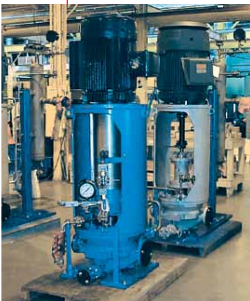
Two-Stage HWM2 Pumps with Oil and Grease Bearing Housings
