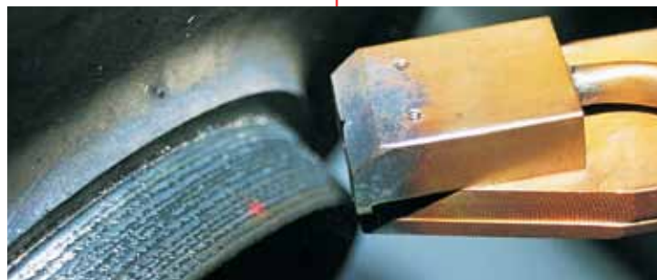
Application of 420 Stainless Steel Powder on CA-15 Impeller Hub
