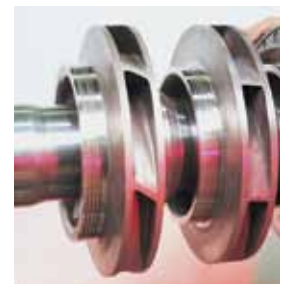
Restored and Upgraded Boiler Feed Impellers
