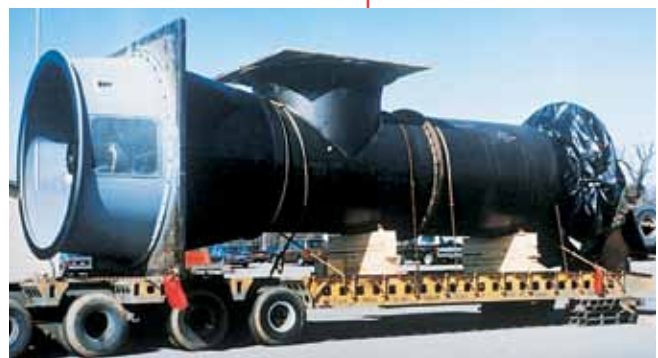
Circulating Water Pump in Silty River Water Service Retrofitted with DLD upgraded shaft sleeves for abrasion and corrosion resistance, highlighted in red.
