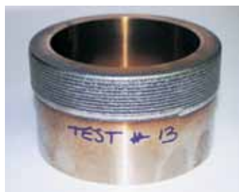
Proof-testing of Ultimet Powder on 316 SS
