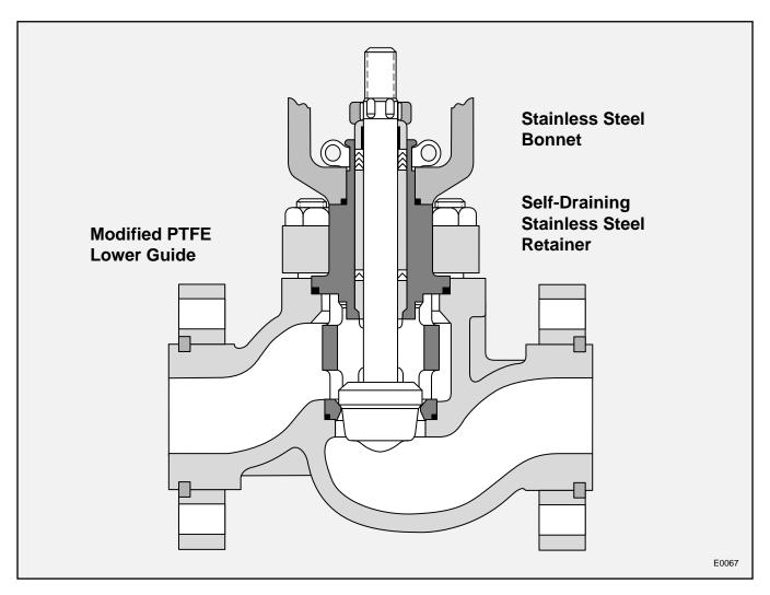
The Valtek® Mark One Sanitary Trim (Mark One-S<sup>™</sup>) valve is a high performance control valve designed to meet the special requirements of the food processing industry. The internal parts of the valve are built with streamlined flow passages, eliminating pockets which could cause fluid stagnation.
