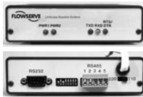
Figure 5.3 – Front and Back Panels of Steered Converter
