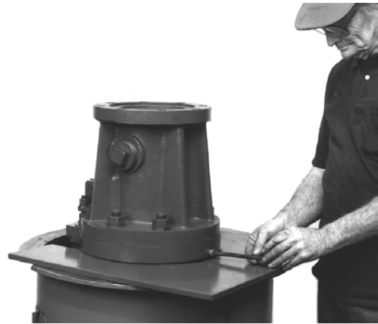
Figure 19 Reinstalling vent plug
