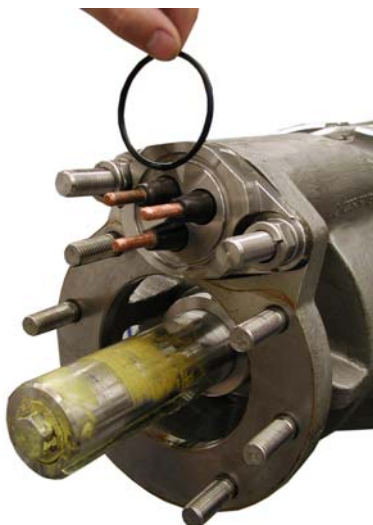
Figure 27 O-ring for metal housing power terminal connector at motor gland plate (4 000 V-cable)
