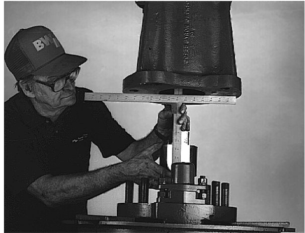
Figure 16 Verify end float
