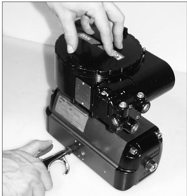
Figure 6: Check Positioner Shaft Alignment
