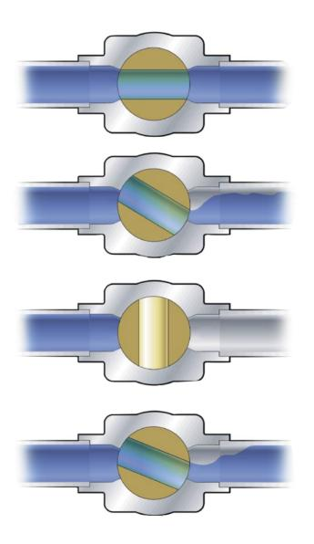
The strength of a Flowserve Nordstrom tapered plug is its seat design. The tapered metal surfaces of the plug and body are fitted together during manufacture using successive steps of turning, grinding and lapping. The result is a nearly perfectly mated metal-to-metal seating surface.
