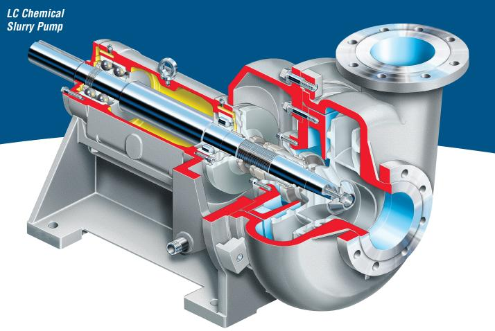
The LC chemical slurry pump is a horizontal, frame mounted, single stage, end suction design with a tangential discharge nozzle. It is available in 26 sizes on only 5 different frames and available in multiple materials of construction to suit application needs. The LC pump is engineered to withstand high concentrations of abrasive and corrosive solutions, like those found in the phosphoric and derived industries as well as mining and mineral processing.
