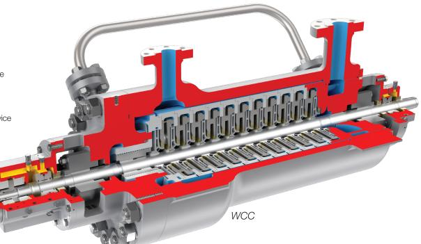
**Multi-vane diffusers** balance radial loads over the operating range while maximizing efficiencies at the duty condition. A continuous metal-to-metal seal between stage pieces minimizes risk of internal leakage.
