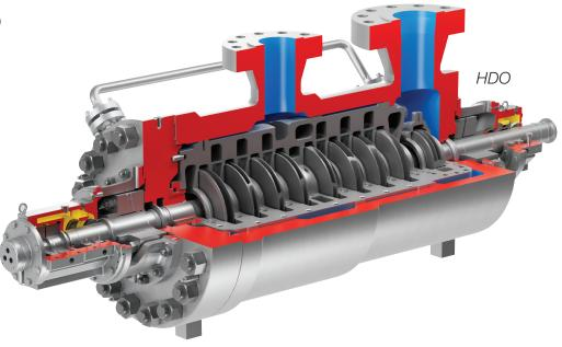
**Double volute casing** consists of two identical halves which feature dual volutes with outlets 180 degrees apart. This design assures radial balance throughout the entire operating range, reducing harmful vibration and ensuring dependable performance.
