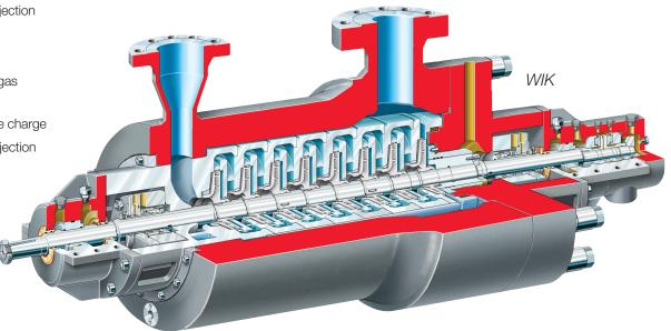
**High-stiffness rotor** with low static deflection is the result of a large-diameter shaft, short bearing spans, unique low specific speed hydraulic designs and high design speeds. This reduces the risk of accidental contact within the running clearances and improves the pump's tolerance to operational upsets.
