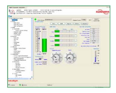
opens a 'window' to the device and allows immediate views with live feedback on all active device sensors including valve stem position, control signal, friction, response time and other important system metrics.
