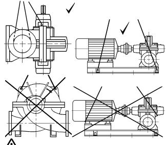
A crane must be used for all pump sets in excess of 25kg (55 lb). Fully trained personnel must carry out lifting, in accordance with local regulations.
