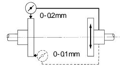
Permissible misalignment limits at working temperature:
