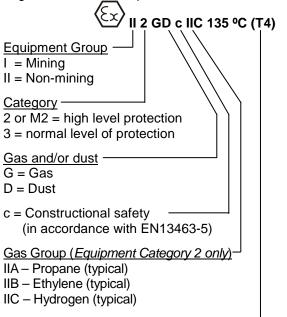
Maximum surface temperature (Temperature Class) (see section 1.6.4.3.)
