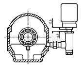
The oil filled bottle should then be refitted so as to return it to the upright position. Filling should be repeated until oil remains visible within the bottle.
