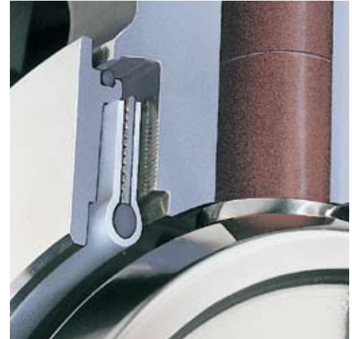
PFA/Viton® A energized seat provides positive, bidirectional shut-off with long cycle life on low pressure and vacuum, and high ΔP services. (See page 23 for more information about seating.)
