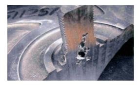
This non-OEM impeller delivered 6 m (20 ft) less head than its intended design. It also did not seal properly to the pump shaft and contained a major shrink void, making it prone to failure in service.
