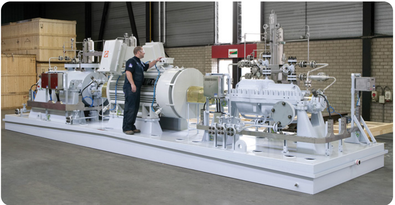
Charge pump train with a 12-stage 6x8x13L HDO barrel pump and an 11-stage 3x10 DMX pump serving as HPRT
