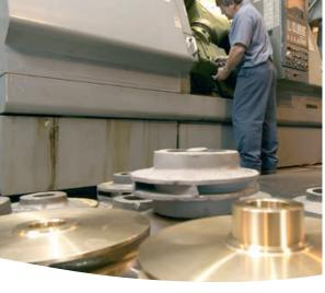
Flowserve Pumps has increased production capacity to meet customer demands for immediate delivery of impellers. Impellers are cast and manufactured to the latest OEM specifications to ensure mechanical integrity, proper metallurgy and high-efficiency performance. Dedicated impeller manufacturing capabilities from Flowserve ensure quick turnaround for the most common pump types and materials to keep your plant running efficiently.
