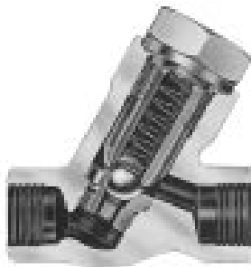
Figure 160: Screwed-Cover, Cover-guided Ball Check, Screwed-in Set
