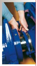
**Removable Stuffing Box** permits easy seal maintenance or seal conversion.
