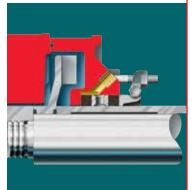
**Optional Expeller Seal** uses centrifugal force to expel fluid from the seal chamber. Recommended for applications in which abrasive particles cause frequent packing failures, clean water is limited, or product dilution is not tolerable.
