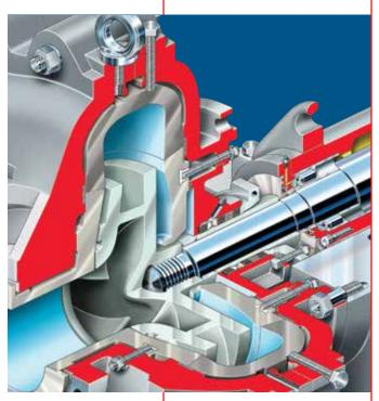
**Captive Metal Liners** are safely handled during in situ rebuilds. The volute is removed while positively clamped into the casing by clamp bolts. Eyebolt meets all lifting safety regulations.
