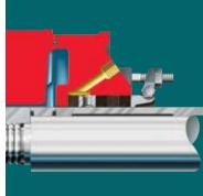
**Gland Packing** is available for most applications. Extra deep stuffing box accepts high-quality gland packing, lantern ring and split gland. Recommended for mineral processing applications in which clean water is available and pump operates in a controlled environment.
