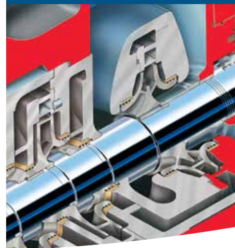
Double-Suction First-Stage Impeller
