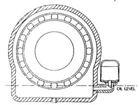
Note: If the pump is fitted with a Constant Level Oiler type "ADAMS", no adjustment of the oil level is possible.
