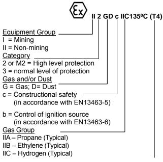
Maximum surface temperature (Temperature Class) (see section 1.6.4.3)
