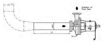
The minimum required straight pipe length (L2) before pump suction inlet is specified in Table 01. The straight pipe section is to be the same diameter as that of the pump suction nozzle.
