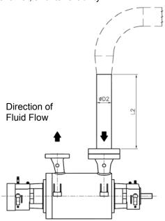
The minimum required straight pipe length (L2) before pump suction inlet is specified in Table 01. The straight pipe section is to be the same diameter as that of the pump suction nozzle.
