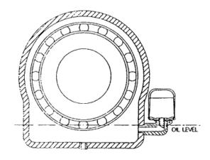
Note: If the pump is fitted with a Constant Level Oiler type "ADAMS", no adjustment of the oil level is possible.
