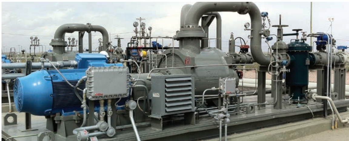
MP1-380 and piping in a single baseplate with separate API Plan 54 seal flush system supplied to Petrobras Energía S.A.
