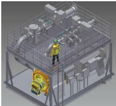
Liquid separator used to maintain stable temperatures in MP1 units running in high-GVF applications or as wet gas compressors
