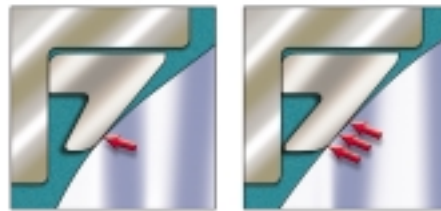
Line contact for low pressure sealing
