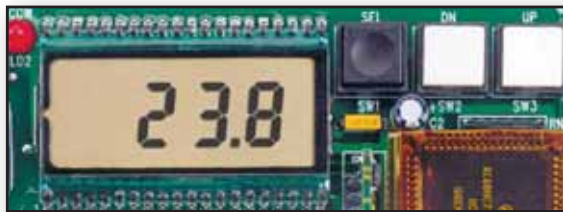
3-button Keypad for on-site calibration and functional set-up
