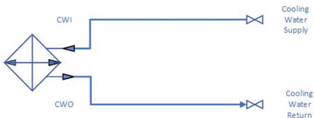
Figure 4: Minimum Cooling Water Piping
