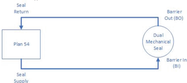
Figure 2 - Minimum Barrier Fluid Piping
