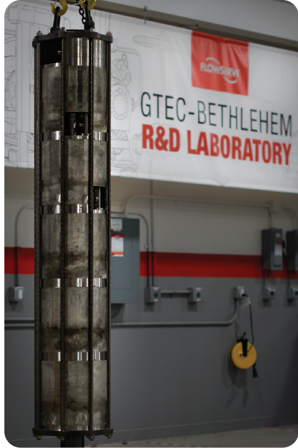
5-Stage Axial Field Integral Motor Pumping System Tie Rod Design
