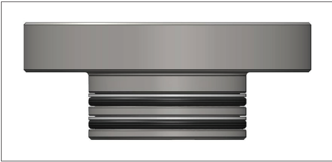
Figure 5: Top Cover with O-Rings and Back-up rings
